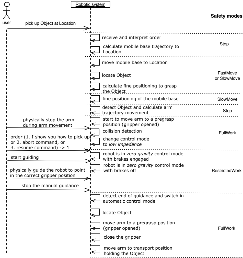
Fig. 4. Sequence diagram of the use case “take an object from a specified location”
