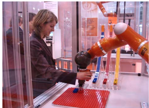
The KUKA Lego cell with the light-weight robot. A visitor is teaching the robot to build Lego brick assemblies.
